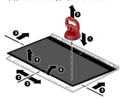
e. To remove the bottom bezel, use a non-marking, non-conductive tool to loosen the bezel from the display (1), rotate the bezel away from the display (2), and then remove the bezel (3).
